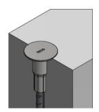
Mount the cap in the socket after removing the nailing plate.
